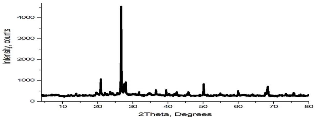
Fig. 4. X-ray diffraction pattern of glauconite sand from the Krantauskoe deposit
